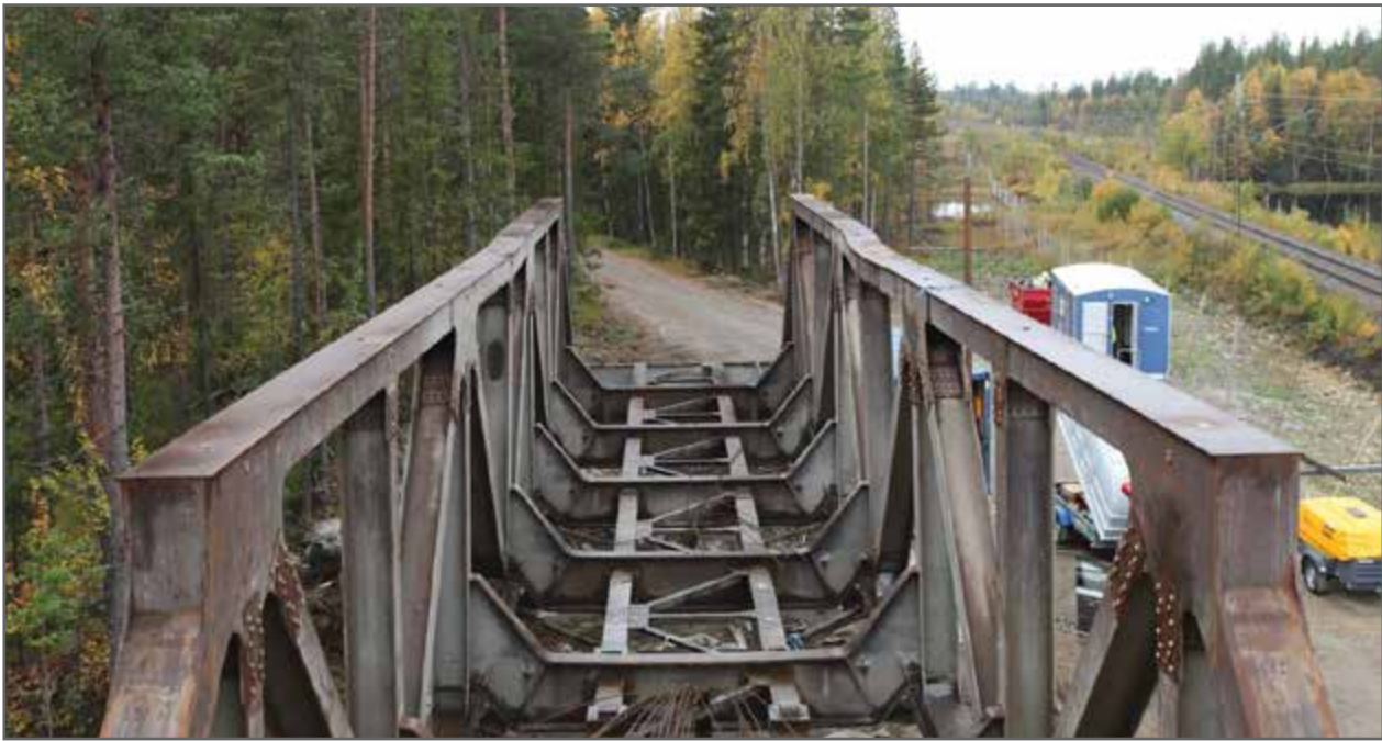
FIGURE 5.4 THE ÅBY BRIDGE AFTER FAILURE. IT WAS CAUSED BY BUCKLING OF THE TOP RIGHT GIRDER. THE FAILURE WAS QUITE DUCTILE AND THE BRIDGE COULD CARRY A HIGH LOAD ALSO AFTER THE MAXIMUM LOAD AS PREDICTED BY THE MODEL IN FIGURE 5-3. A PART OF THE FEM MODEL OF THE FAILURE IS SHOWN IN THE INSERT. © MAINLINE CONSORTIUM
